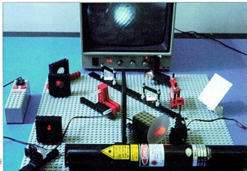
Mach Zehnder patterns: the Lego interferometer produces fringes on the screen (right) and on the rotating ground-glass screen imaged by the camera and presented on the monitor.
